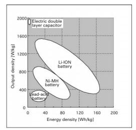
Energy density: the amount of electrical power the unit can produce in one hour Output density: The maximum instantaneous electrical output
