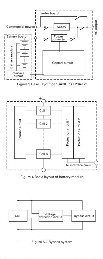
the inverter. During normal operation, only the "quality" component is handled by the inverter. Compared with consistent inverter supply, this method has less power loss and can thus supply power to the load more efficiently. If there is a problem with the commercial power supply, the device immediately switches off of the commercial power supply and the power converter begins to
